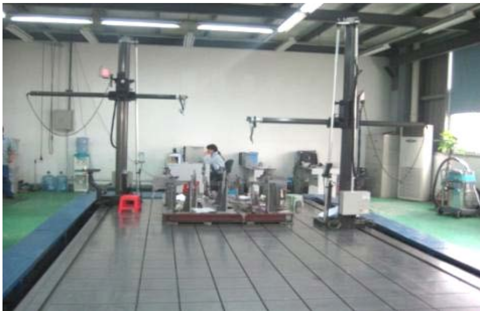
平台式三坐标 Platform three coordinates
